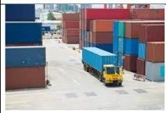
Terminal tractors are semi-tractors used to move containers on semi-trailers within a cargo yard, warehouse facility, or intermodal facility. Also known as shunt trucks, spotter trucks, spotting tractors, utility tractor rigs (UTRs), **yard trucks**, yard tractors, yard shifters, yard birds, yard dogs, yard goats, yard horses, yard jockeys, and mules.
