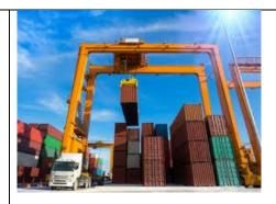
Rubber-tired gantry (RTG) cranes use a cross-beam supported on vertical legs that move on rubber tires to move and stack loaded containers. A rail-mounted gantry (RMG) crane is similar to an RTG and typically used in larger operations.
