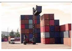
Side handlers use an overhead telescopic boom to lift and move cargo containers sideways by "grabbing" the sides or top and bottom of the longest side of a container. They are used to move and stack empty containers.
