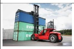
Top handlers use an overhead attachment on a straight mast to move and stack loaded containers. They can be used in place of or in conjunction with RTGs to lift heavy containers within a terminal. Also known as top loaders, top picks, top lifts, and loaded container handlers.
